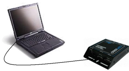
COM1000 connected to a PC using a crossover cable
