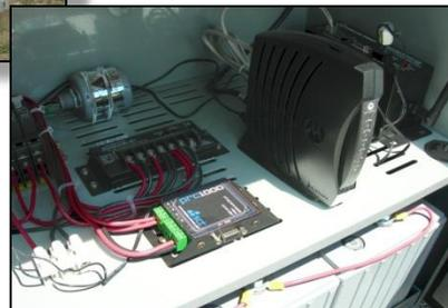
PRC1000 controls power to both the cable modem and the wireless radio on a regularly scheduled basis.
